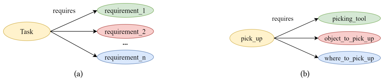
Figure 1: Task definition structure: (a) General structure; (b) Example of task definition for a “pick_up” task.
