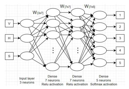
Figure 13: Architecture of the Neural Network with Two Hidden Layers
