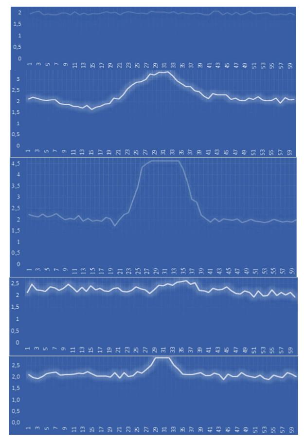
**Figure 3:** Graphs of the training dataset: a – Absence of a mine, b – Anti-tank mine, c – Antipersonnel mine, d – Booby trap mine, e – M14 mine, where x – sensor position (cm) and y – anomaly voltage (V) [6]
