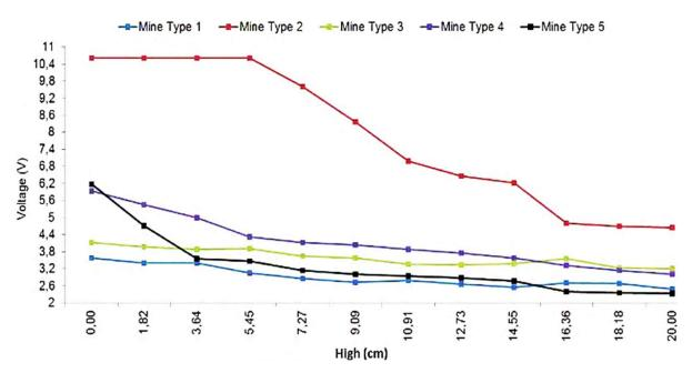
Figure 2: Magnetic field anomaly values relative to depth for each mine type [6]
