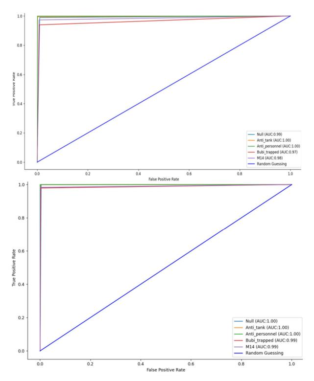
**Figure 15:** ROC Curves for Each Type of Mine, where a – Neural network with one hidden layer, b – Neural network with two hidden layers.
