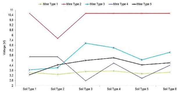
Figure 1: Magnetic field anomaly values relative to soil type for each mine type [6]
