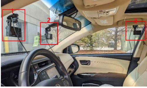
Figure 2: Camera mounting setup for the three views in the SynDD1 dataset: 1. Dashboard, 2. Behind rear view mirror, and 3. Top right side window.
