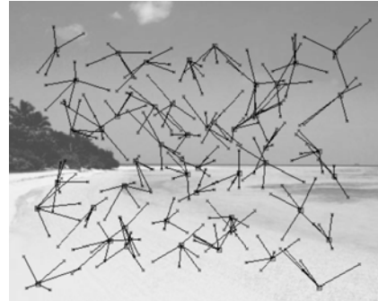
Fig 3 : A space-variant logarithmic ( R0=2 ) retina for TheVibe. Note that the extent of the receptive fields increases with eccentricity. In particular, our mapping preserves overlap.
