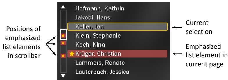
Fig. 4. Three elements are emphasized in a selection list by the List Item Emphasis pattern. The emphasized elements are supposed to be selected more frequently by the user than others.
