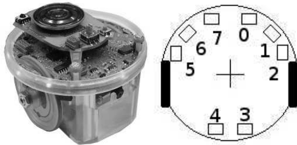
Fig. 1. Miniature e-puck robot has eight infrared sensors and two motors.
