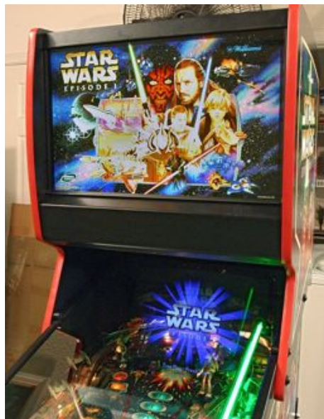
Figure 29 Star Wars Episode I , showing the reflection of the top-mounted monitor on the combining mirror over the rear/upper playfield. Photo by Allen Shope.
