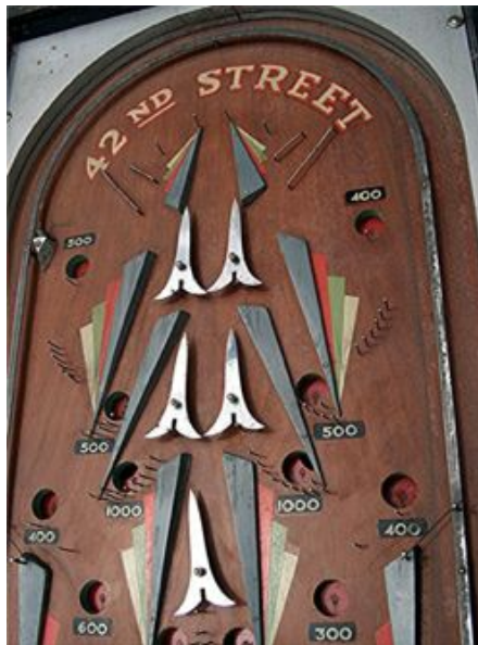
Figure 3 Diverters on this table affect the path of subsequent shots (Genco ‘42 nd Street’).
