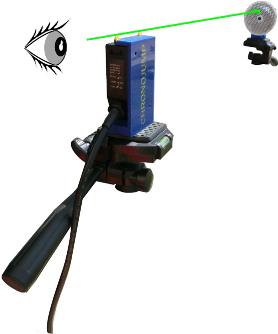
Figura 12.1: Alignment of the photocell
