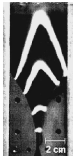
Fig. 3. Example of dynamic discharge in a sliding arc non-thermal plasma reactor (Copyright Elsevier [74]).
