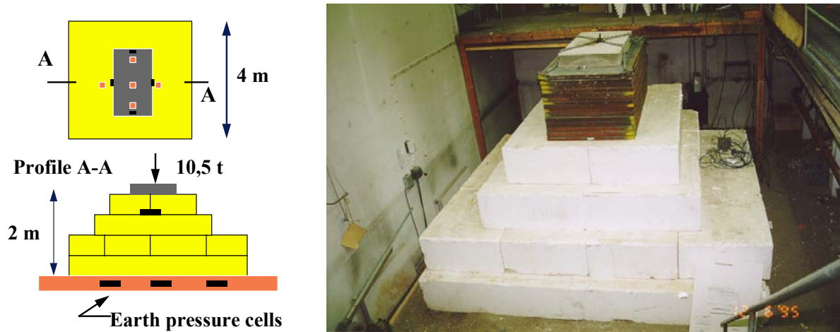
Figure 8. EPS test fill at the Norwegian Road Research Laboratory (now the Road Technology Department).
