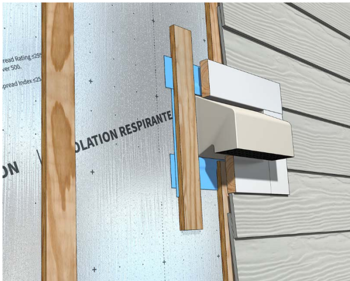
Step 3 - Install furring strips prior to cladding, trim installation
