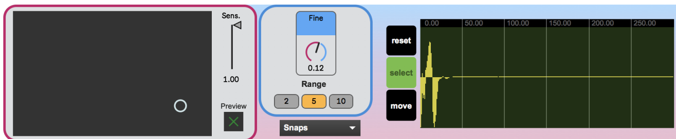
Figure 5: The Neural Drum Machine interface. First, the XY pad on the left controls values for the two most influential dimensions. The "Fine" knob controls the value for the third most influential dimension and can be seen as fine tuning. The range selector controls the range of values available for these three dimensions. Then, a selector allows the user to control which type of sound is generated. Finally, the waveform visualizer on the right allows to trim a sample to play only a particular region.
