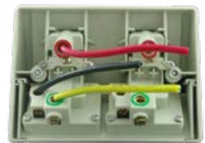
Separate Switch Wiring
