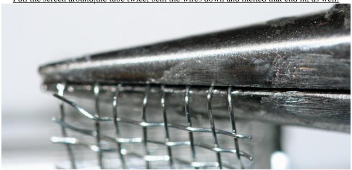
Melt some wire into the end and trim, making 3 or 4 wires to keep up off the base.
