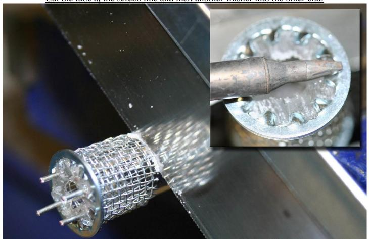
With pliers, bend a piece of wire, as shown, and melt it into the top.
