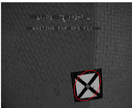
Fig. 7. Example marker detection results in real-life captured image
