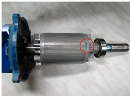
Fig.1.c) Rotor of TPIM with 2 broken bars.
