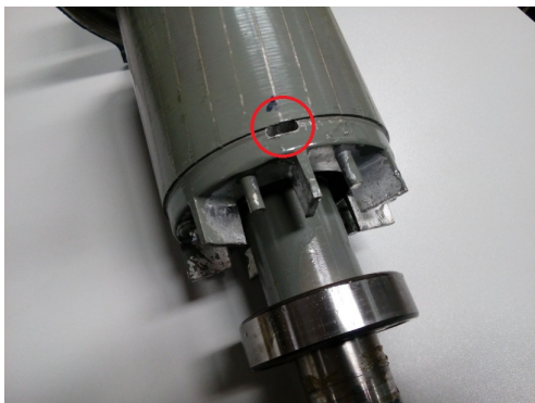
Fig.9.b) Squirrel cage of the TPIM with one broken bar.
