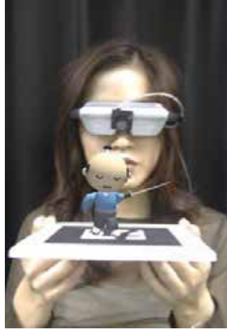
Figure 10. AR with head mounted display and 3D graphic placed on fiducial marker (Billinghurst, Poupyrev et al. 2000)
