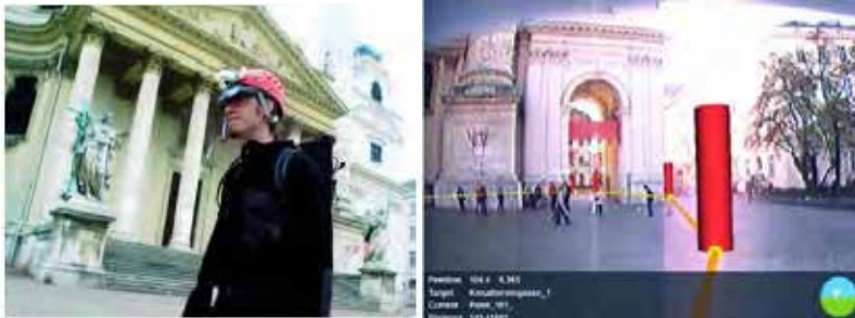
Figure 15. Mobile AR tour guide system (left) and AR display of path to follow(right) (Reitmayr and Schmalstieg 2004)
