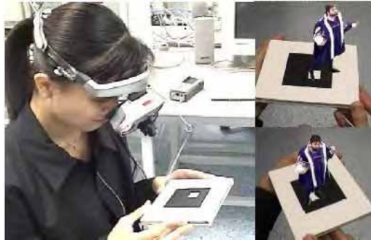
Figure 12. Remote collaborator as seen on AR fiducial marker (Prince, Cheok et al. 2002)
