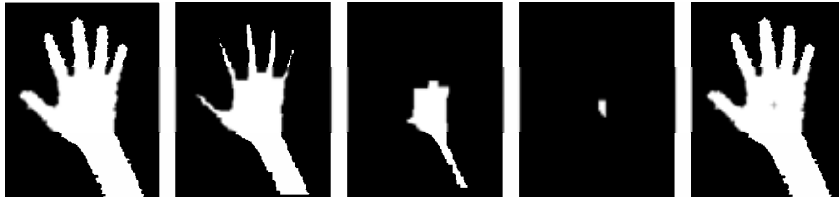
Figure 8. Procedure for finding the center of the palm by the morphological erosion operation
