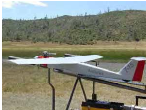
Figure 8: The Arcturus T-15 airframe and launcher
