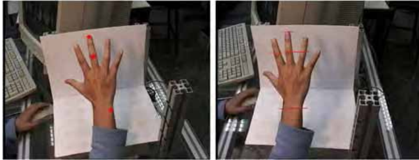
Figure 17. Find corresponding points in the right image which are marked by red points, for points in the left image which are marked by red crosses, using the color correlation and epipolar geometry
