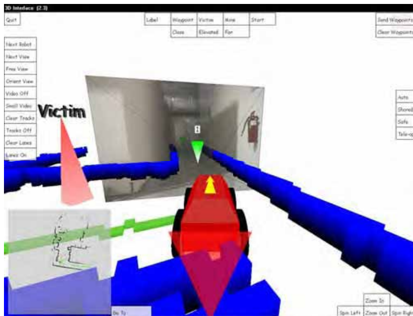
Figure 5. Interface showing fusion of video and map representation
