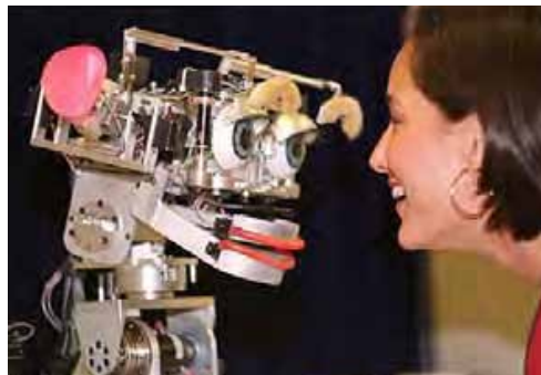
Figure 7. Kismet showing facial expressions present in human communication (Breazeal, Edsinger et al. 2001)
