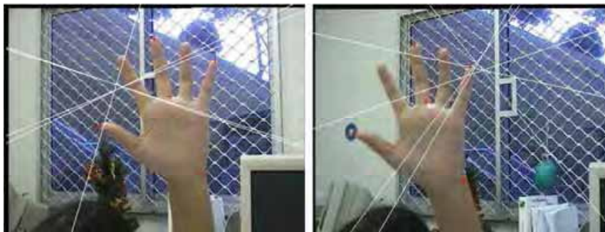
Figure 15. (a) Extracted matches using the method proposed by Zhang from uncalibrated hand images shown in Fig. 13, (b) Estimated epipolar geometry from these matches
