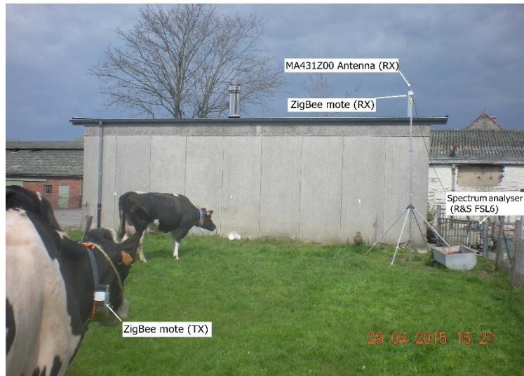
644 Fig. 3. Measurement setup of the second scenario: environment with cows and setup with ZigBee 645 mots.
