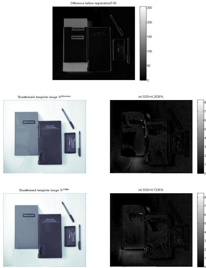
FIGURE 3. Registration results for two book images of size 512 \times 512 (Example 2). Top row: Difference between reference image and template image before registration. Middle row left: registered template image by \mathcal{R}^{\text{NewC}} ; Middle row right: Difference between reference image and deformed template image after registration by \mathcal{R}^{\text{NewC}} ; Last row left: registered template image by \mathcal{R}^{\text{CCBc}} ; Last row right: Difference between reference image and deformed template image after registration by \mathcal{R}^{\text{CCBc}} . Here the heuristically best \alpha were selected for all cases and \beta = 10^{-6} .
