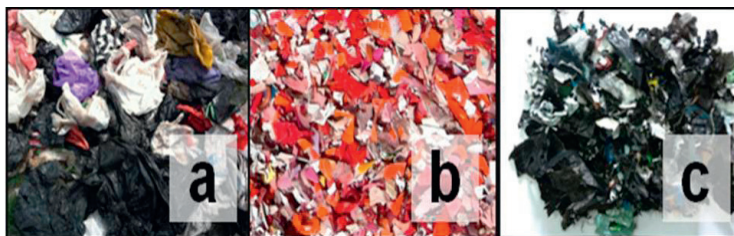
Fig. 1. The feedstock used in the experiments : (a) PE bag 1; (b) HDPE waste; and (c) PE bag 2.
