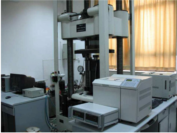
Fig. 19. Experimental system for mechanical properties of deep rocks under high temperature.
