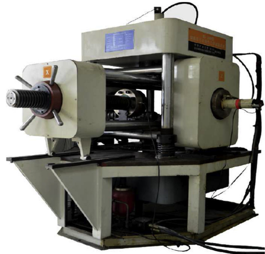
Fig. 23. Impact rockburst experiment system (He et al., 2013).
