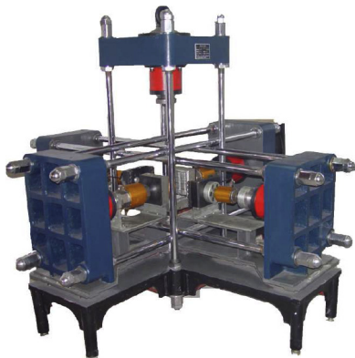
Fig. 22. Strain rockburst experiment system (He et al., 2012a,b).
