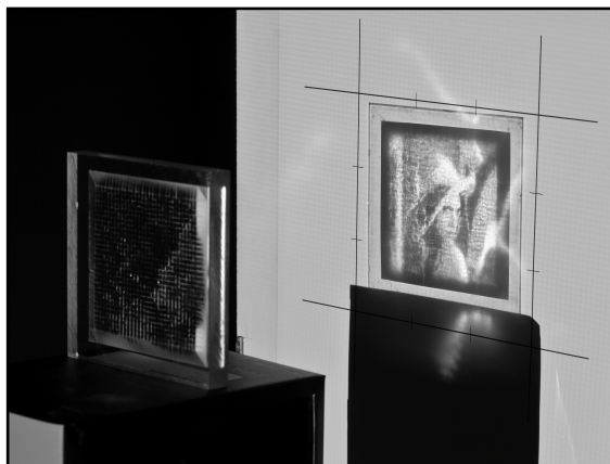
Figure 1: We design and mill piecewise-smooth arrays of micropatches which reshape incident light onto a collection of Gaussian caustics, to approximate arbitrary images at a projection plane. Above, we show a photograph of a physical sample projecting the Lena image.
