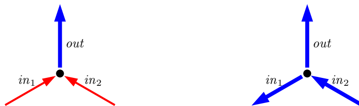
■ Figure 2 Two types of nodes. Edges with weight 1 are shown in red and edges with weight 2 are shown in blue. Left: An AND node. The minimum in-flow requirement of the vertex is 2. Edge out can be directed outwards only if both in 1 and in 2 are directed inwards, if the minimum in-flow constraint were to be maintained. Right: A protected OR node. Edge out can be directed outwards if either in 1 and in 2 is directed inwards. In a protected OR it is not possible for both in-edges to be directed inwards simultaneously.
