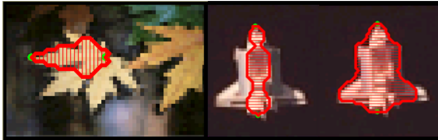
FIGURE 36. The leaf image on the left shows how the extensive nature of the energy can force a simplification of the topology. In addition to the green dots in the image, there were four more terminal points at the tips of the leaf lobes. Skipping has allowed the model to find only a one-part region. The two right hand images show the effect of increasing the area term. The co-circularity energy itself has a tendency to make the region found slimmer. The balance between this term, the extensive nature of the energy and the area term is complicated.
