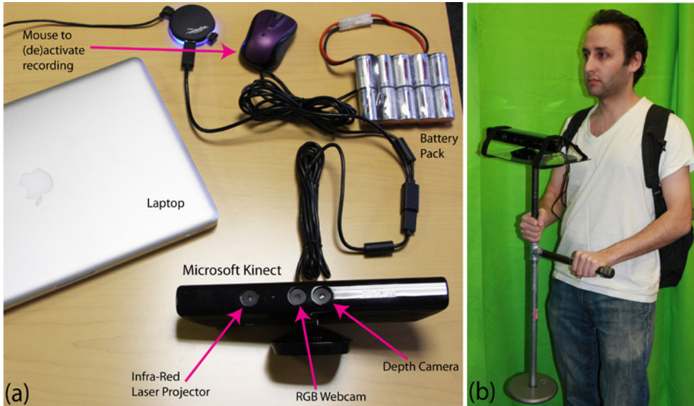
Figure 3.2: (a): Our capture system with a Kinect modified to run from a battery pack. (b) Our capture platform, with counterweights to damp camera movements.
