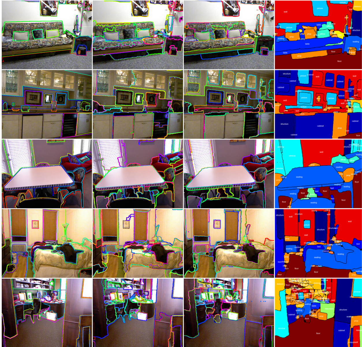
Figure 5.5: Random test images from the NYU Depth V2 dataset, overlaid with segmentations. 1st column: ground truth. 2nd column: segmentations from Jia et al [19]. 3rd column: our segmentations. 4th column: semantic labels, produced as a by-product of our segmentation procedure.
