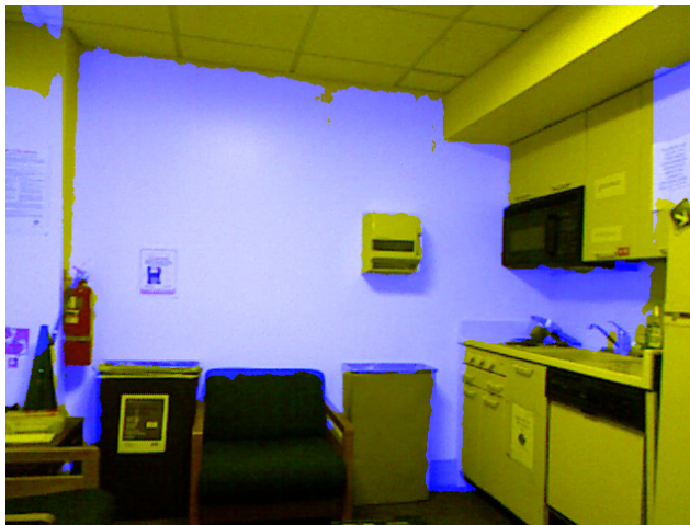
Figure 4.2: A demonstration of our scheme for finding the boundaries of the room. In this scene, the blue channel has been replaced by a binary mask, set to 1 if the depth of point is within 4% of the maximum depth within each column (and 0 otherwise). The walls of the room are cleanly identified, while segmenting objects of similar depth such as the fire extinguisher and towel dispenser. On the right, the cabinets and sink are correctly resolved as being in the room interior, rather on the boundary.
