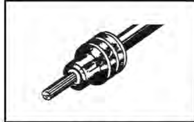
2. Align seal with cable insulation.
