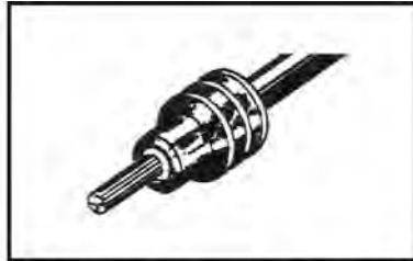
2. Align seal with cable insulation.
