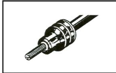
2. Align seal with cable insulation.
