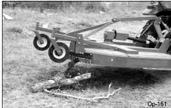
Raise Mower over solid objects
