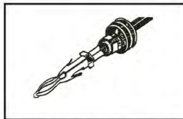
4. Crimp and visually inspect for a good crimp before installing in connector body.
