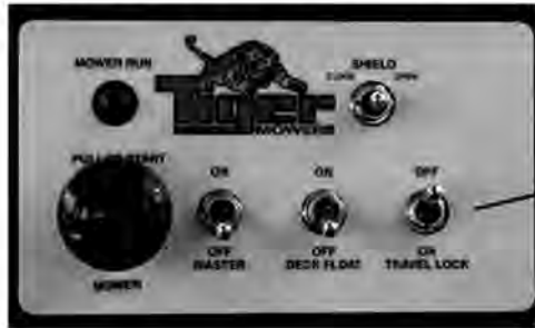
ELECTRONIC LIFT VALVE SWITCH BOX
