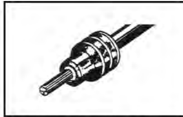
2. Align seal with cable insulation.
