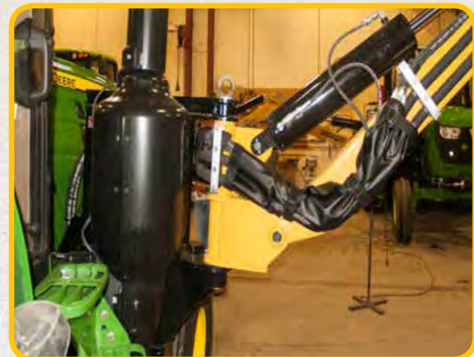
Connection complete - back side view. Approx. 4 hrs shop time to complete assembly.
