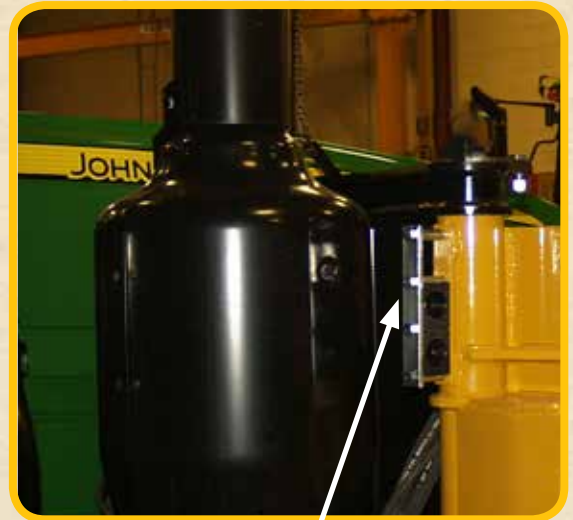
Attach hose clamp to side of swivel.
