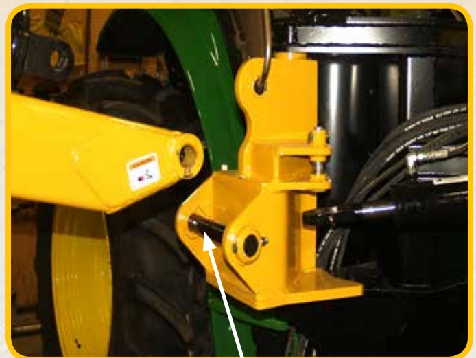
Connect end of primary boom arm to swivel with horizontal pin. Total time for assembly is 1 1/2 hours.
