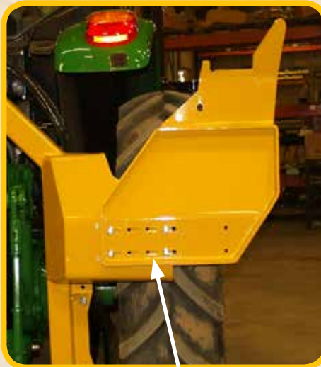
Take out 4 bolts in stow plate and slide to far right, this is the working position for stow.
