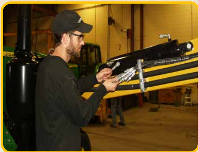
Attach 1/4" lines so that controls can be used to help lift and line up boom arm fitting.
