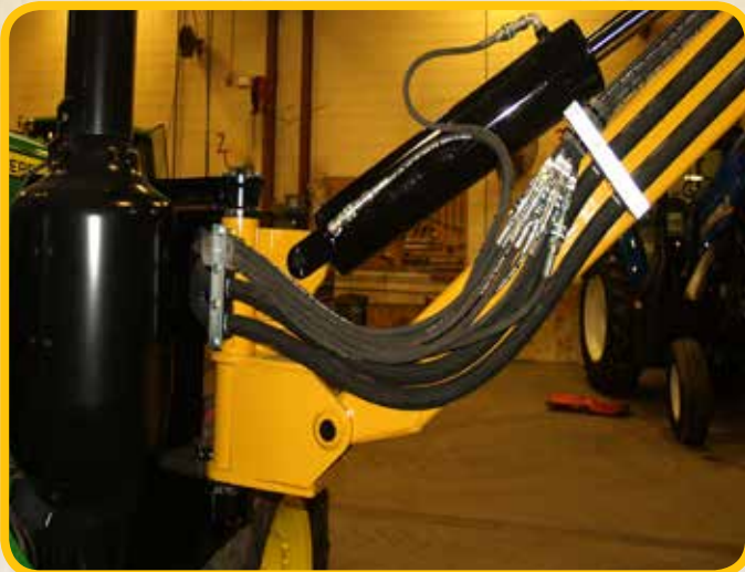
Run 1" lines on bottom 2 spaces of clamp and run 1/4" lines on top space. Measurement is 38" for 1" lines, clamp to clamp. Match 1/4".
