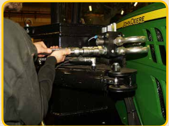
Connect 1" hoses. Wrap hoses in teflon wrap. Wrap is located in the cab of tractor.
