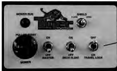
ELECTRONIC LIFT VALVE SWITCH BOX
