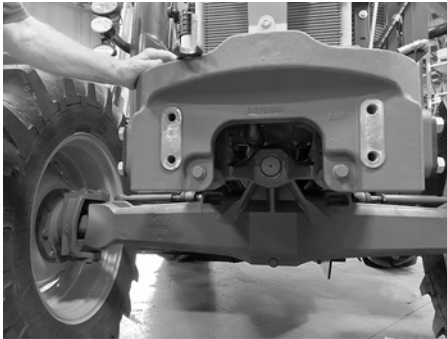
The bolster on the front of the tractor must be temporarily removed.
