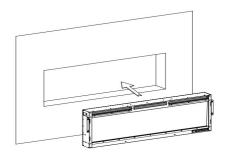
**4.A5)** Fix the firebox with screws(BB). on the side wood stud by a Phillips screwdriver (not included).
