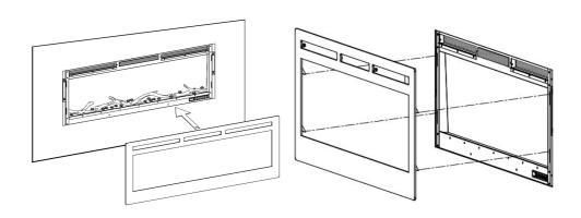
4.A10) Fix the glass front by screws (CC) and complete the installation. Screws (CC) reference model configuration.
