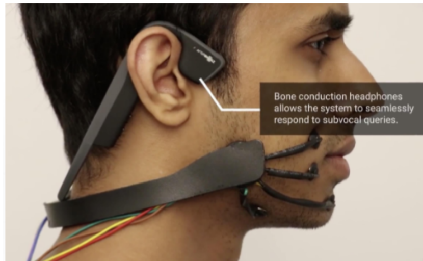
Figure 6. Bone conduction aural output of the AlterEgo system, making it a closed-loop input-output platform.
