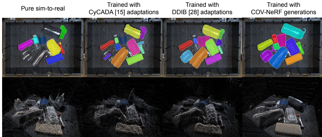
Figure 5.5: Sample instance segmentation predictions from MaskDINO (top row) and stereo depth predictions from MVS-Former (bottom row) resulting from the sim-to-real methods evaluated in Table 5.3. COV-NeRF enables substantial improvement in both modalities.
