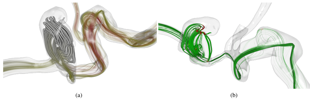
Figure 3: Different parameter mapping options for pathlines. In (a), the residence time inside the aneurysm is mapped to the opacity and the flow velocity is mapped onto color using a temperature scale (white is slow). In (b), the per-vertex fitness indicator is mapped to color (green-to-red-scale) and the overall line fitness is mapped to thickness.
