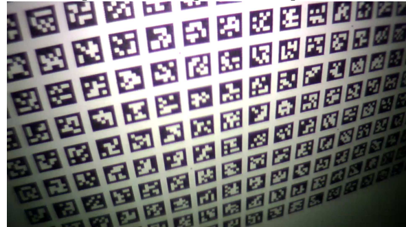
Figure 5. The 216 tag AprilTag calibration pattern.
