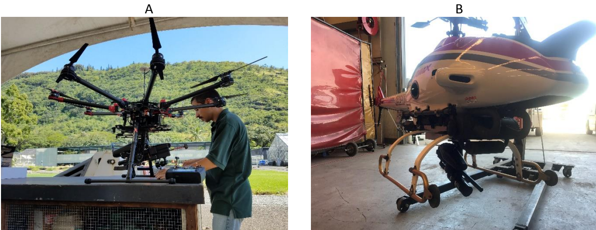
3. (A) Graduate Student Roberto Rodriguez installing the HBT gimbal platform to the S-1000 ® octocopter (DJI Co., Ltd, Shenzhen, China) and (B) HBT gimbal installed on the Rmax ® heavy-lift UAS (Yamaha Motor Corp. USA, Cypress, CA) in collaboration with Dr. Ken Giles (UC Davis).
