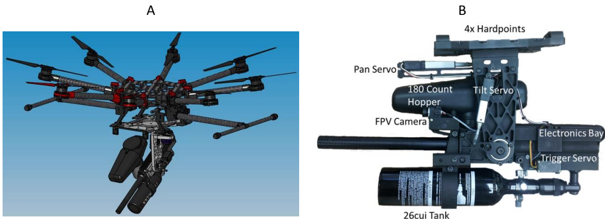
Figure 1. (A) CAD rendering of the HBT-UAS design. (B) Side view of gimbal-marker system.
