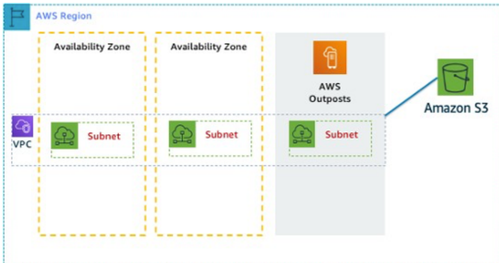
Example AWS Outposts architecture
