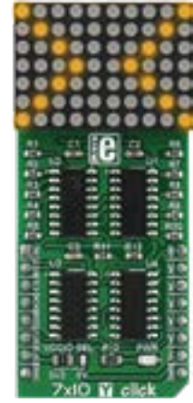
7x10 Y Click With a matrix of 70 yellow LEDs driven by a pair of 8-bit serial-in, parallel-out shift registers. MSRP - $15 00 MIKROE-2790
