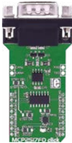
MCP2517FD Click With MCP2517FD CAN FD controller and ATA6563 high-speed CAN transceiver. MSRP - $25 00 MIKROE-2379
