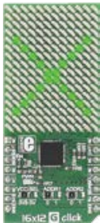
16x12 G Click Carries a 16x12 LED display and the IS-31FL3733 matrix driver with 1/12 cycle rate. MSRP - $30 00 MIKROE-2758
