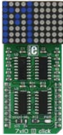
7x10 B Click With a matrix of 70 blue LEDs driven by a pair of 8-bit serial-in, parallel-out shift registers. MSRP - $15 00 MIKROE-2789
