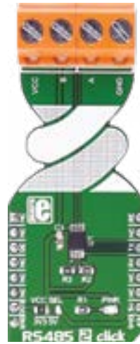
RS485 2 Click Carries MAX3471 half-duplex transceiver for lithium battery-powered RS-485/RS-422 applications. MSRP - $18 00 MIKROE-2700
