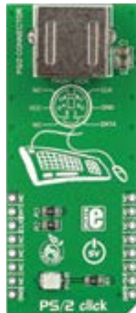
PS/2 Click Adds keyboard and mouse connectivity. With a standard 6-pin Mini-DIN PS/2 connector. MSRP - $9 00 MIKROE-1576
