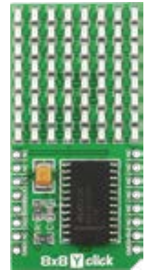
8x8 Y Click It features MAX7219 8-digit LED display driver module as well as 64 YELLOW LEDs. MSRP - $15 00 MIKROE-1294
