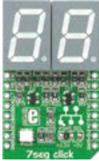
7seg Click 2-digit seven-seg display. With two 74HC595 8-bit serial-in, parallel-out shift registers. MSRP - $10 00 MIKROE-1201
