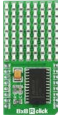
8x8 R Click It features MAX7219 8-digit LED display driver module as well as 64 RED LEDs. MSRP - $15 00 MIKROE-1295
