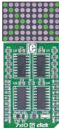
7x10 G Click With a matrix of 70 green LEDs driven by a pair of 8-bit serial-in, parallel-out shift registers. MSRP - $15 00 MIKROE-2705
