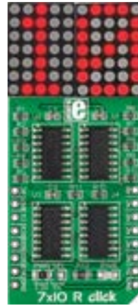
7x10 R Click With a matrix of 70 red LEDs driven by a pair of 8-bit serial-in, parallel-out shift registers. MSRP - $15 00 MIKROE-1993
