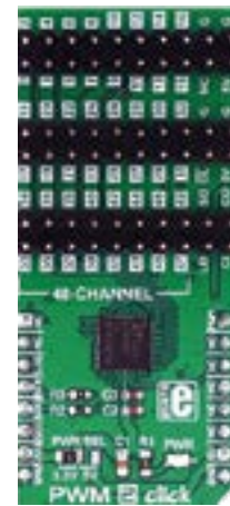
PWM 2 Click With the LT8500, a 48-Channel LED PWM generator with 12-Bit res. and 50MHz serial interface. MSRP - $27 00 MIKROE-3148
