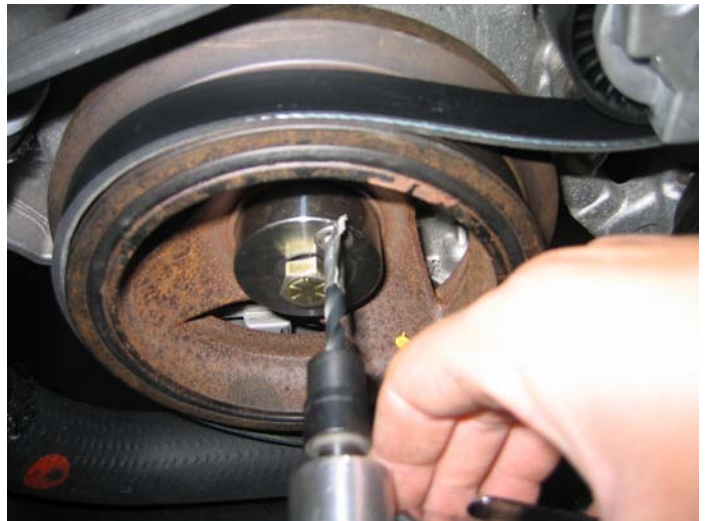
Drilling the Crank
