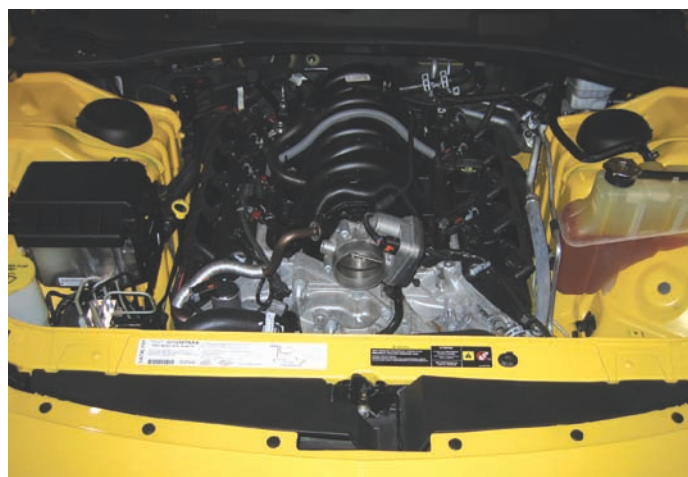
Engine Air Filter Removed
