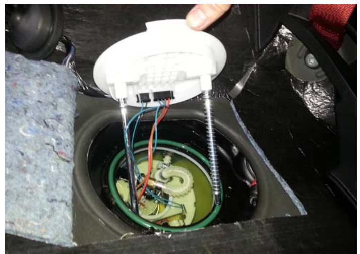
Electrical Connectors Under Pump Lid
