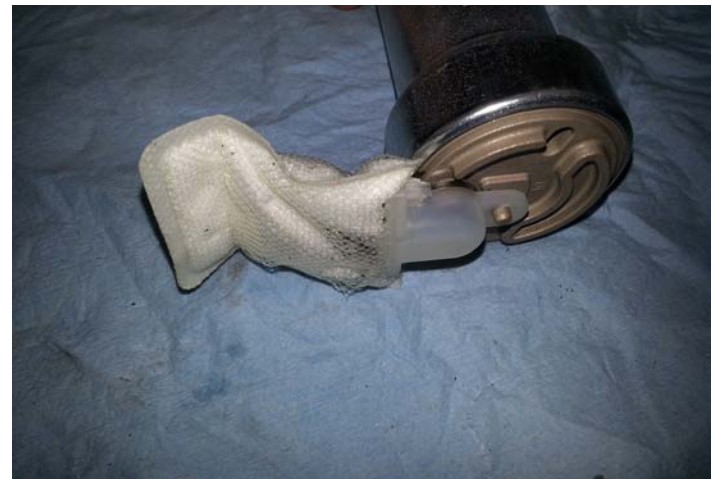
New Fuel Sock Installed
