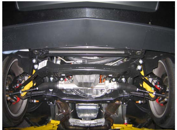
Underside Body Cladding Removed
