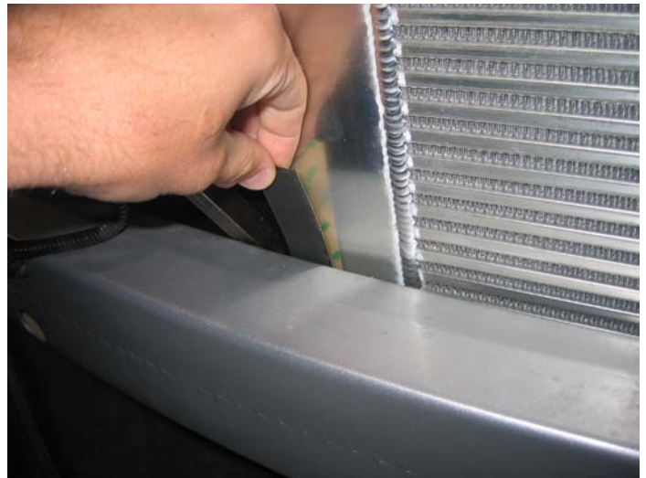
Place Tape Between Intercooler and Front Bumper for Insulation
