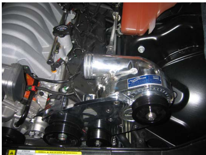
ProCharger Head Unit Installed
