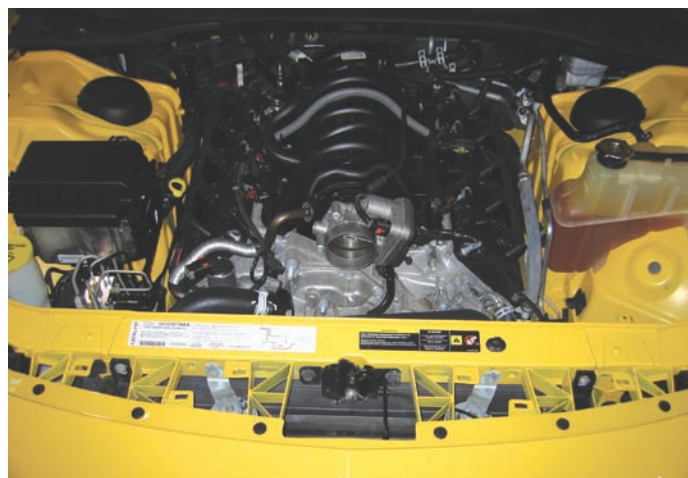
Radiator Cavity Covers Removed
