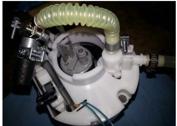
Jet Siphon Installed in Basket
