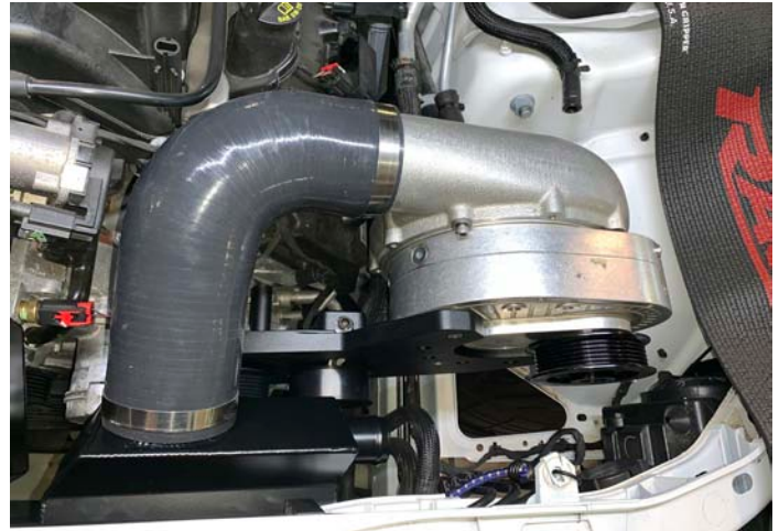
Tube and Reducer Installation
