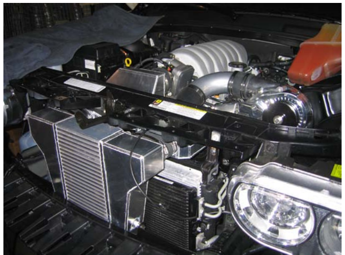
Intercooler and Tubing Installed
