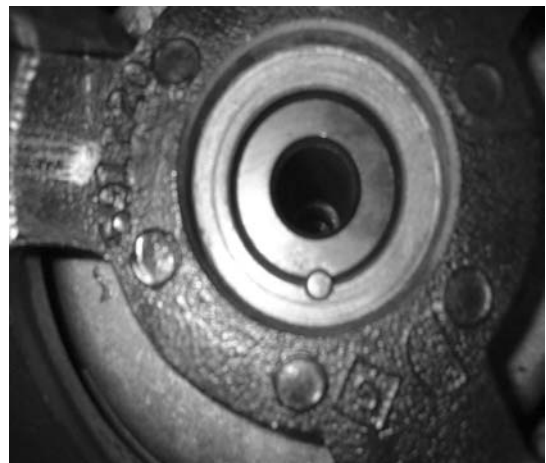
Crank Pulley Pinned to Crankshaft
