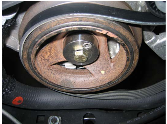
Drill Jig Installed
