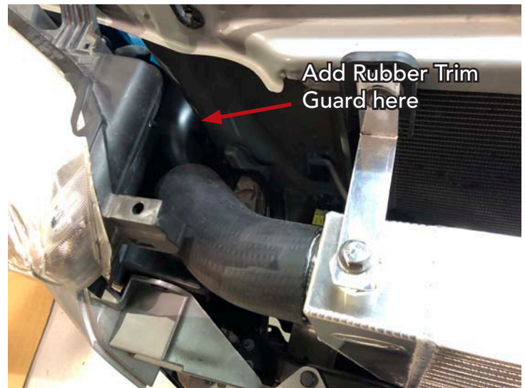
Tubing Out Of Intercooler Installed
