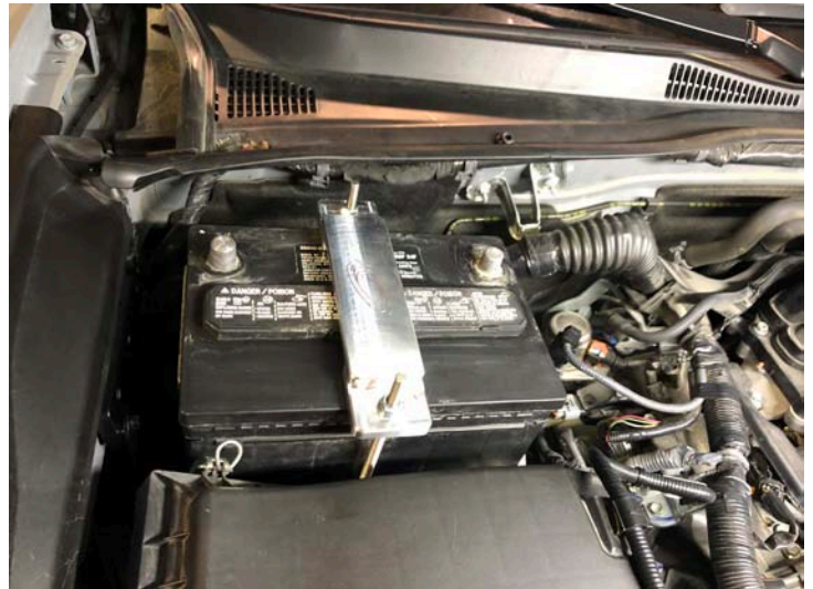
Battery Hold Down Installed
