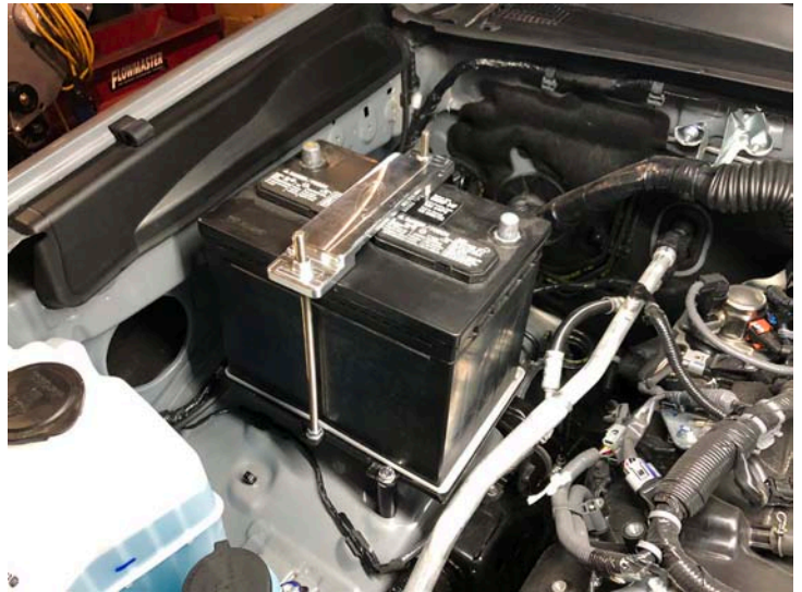
Battery And Hold Down Installed
