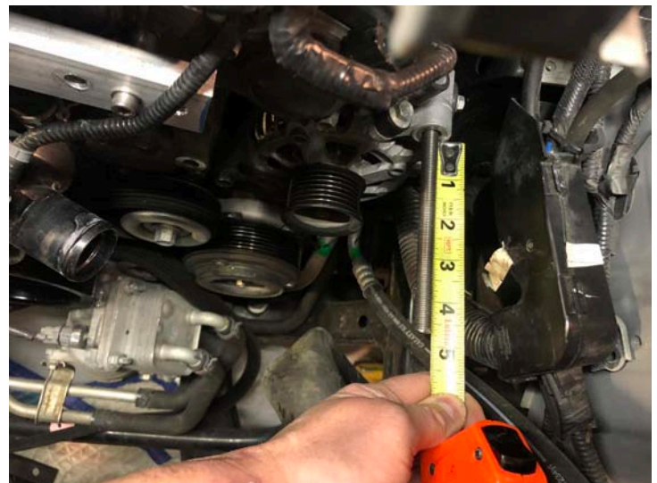
Alternator All Thread Installed
