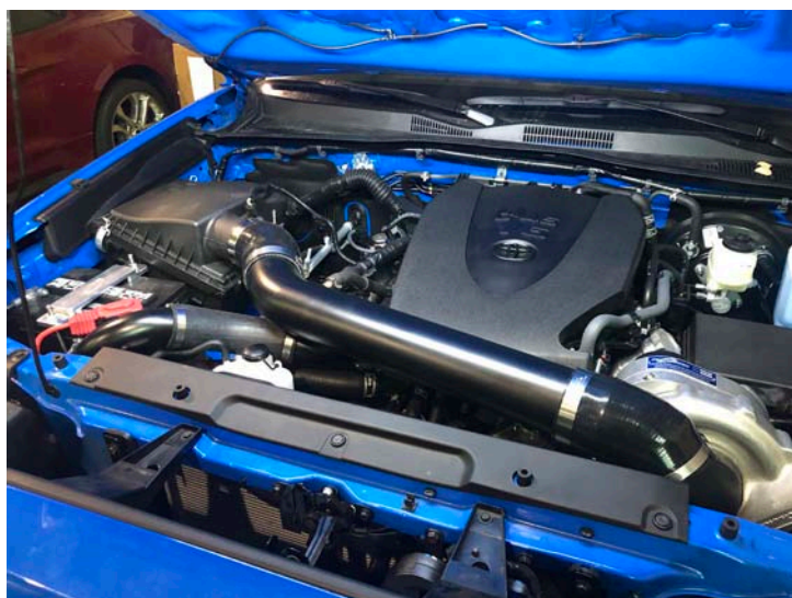
Air Inlet Tube Installed
