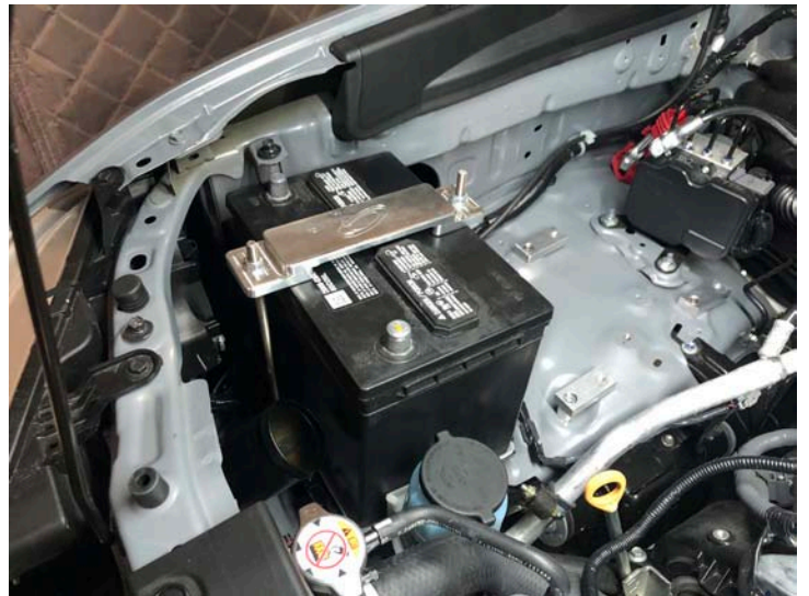
Battery Hold Down Installed
