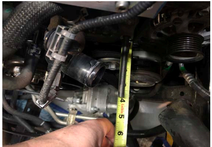
Idler All Thread Installed
