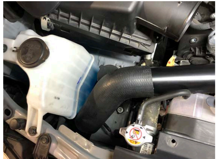
70° Rubber Elbow Installed
