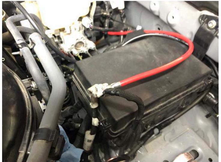
Positive Battery Cable Installed
