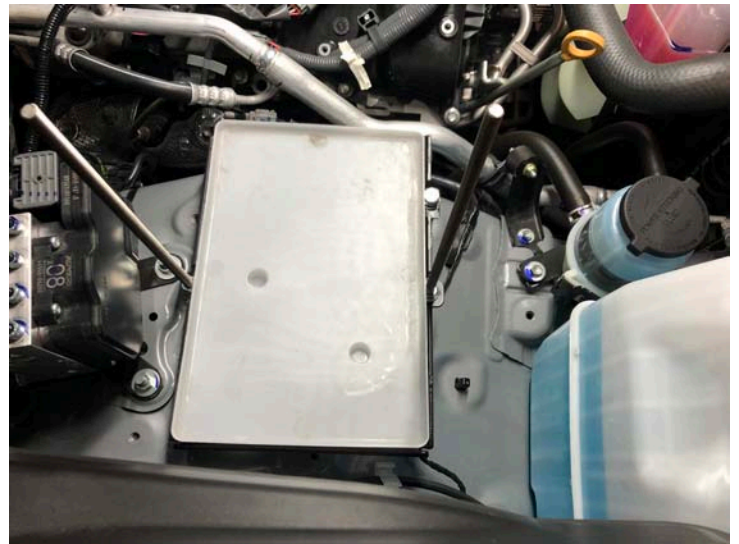
Plastic Battery Tray Installed
