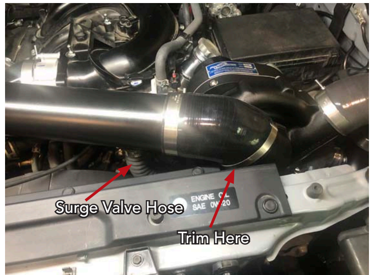
Inlet Tubing Connected To Supercharger
