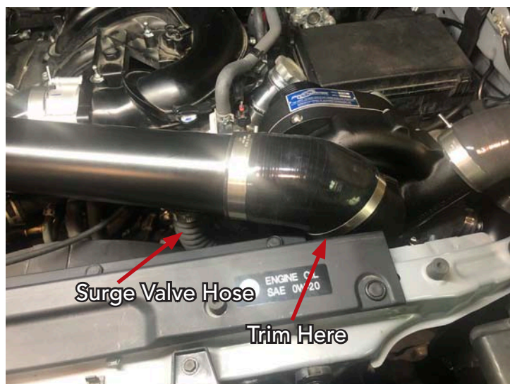
Inlet Tubing Connected To Supercharger
