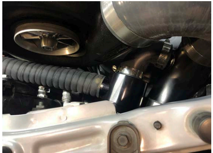
Surge Valve And Flexible Hose Installed
