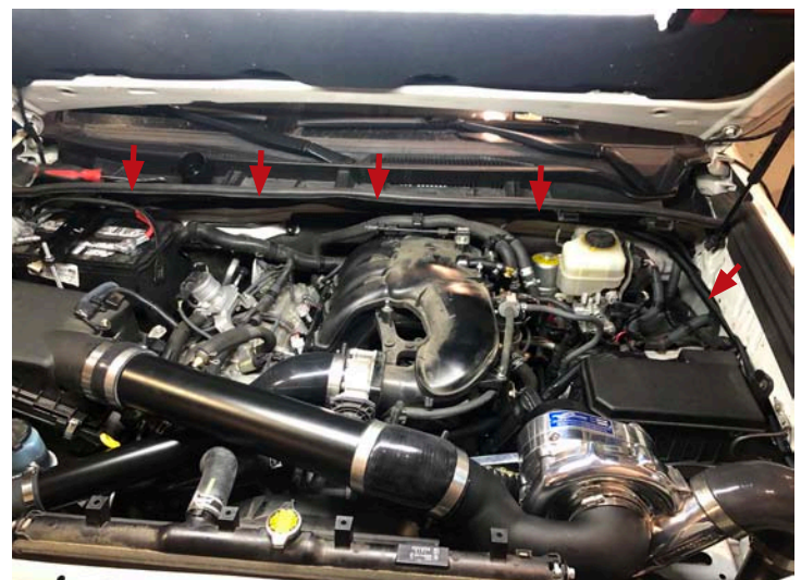
Battery Cables Routed
