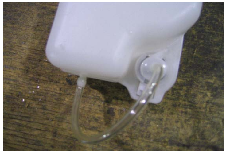
Windshield Washer Hose Routing
