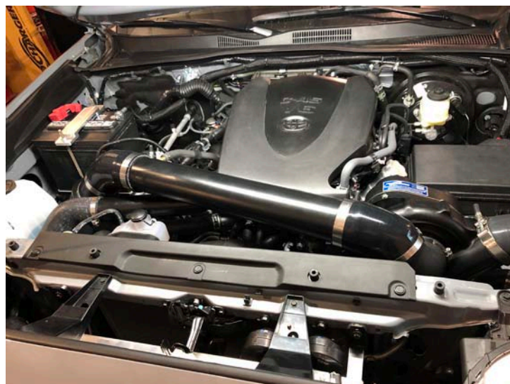
Air Inlet Installed
