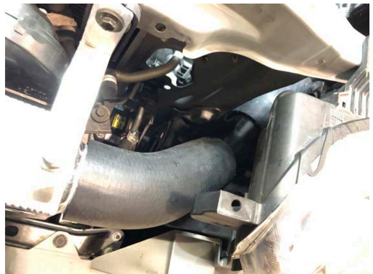
Tubing To Intercooler Installed
