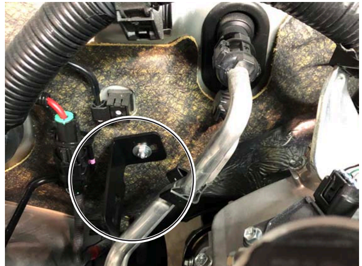
"L" Bracket Installed
