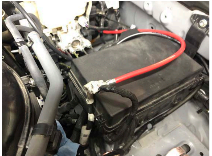
Positive Battery Cable Installed
