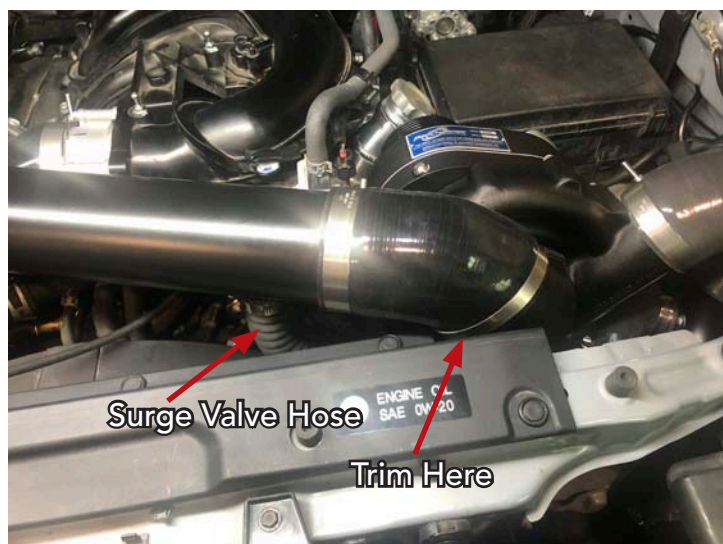
Inlet Tubing Connected To Supercharger
