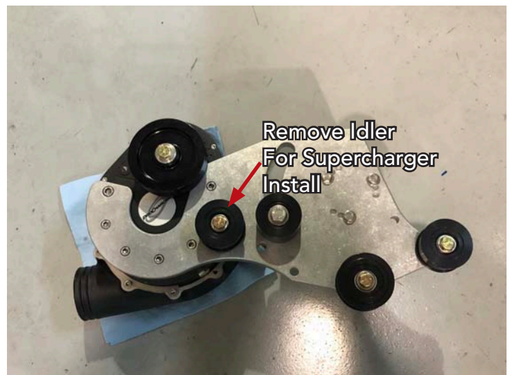
Supercharger Installed Onto Bracket
