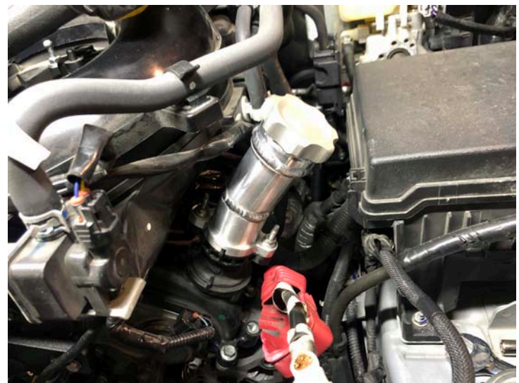
Oil Fill Neck Installed
