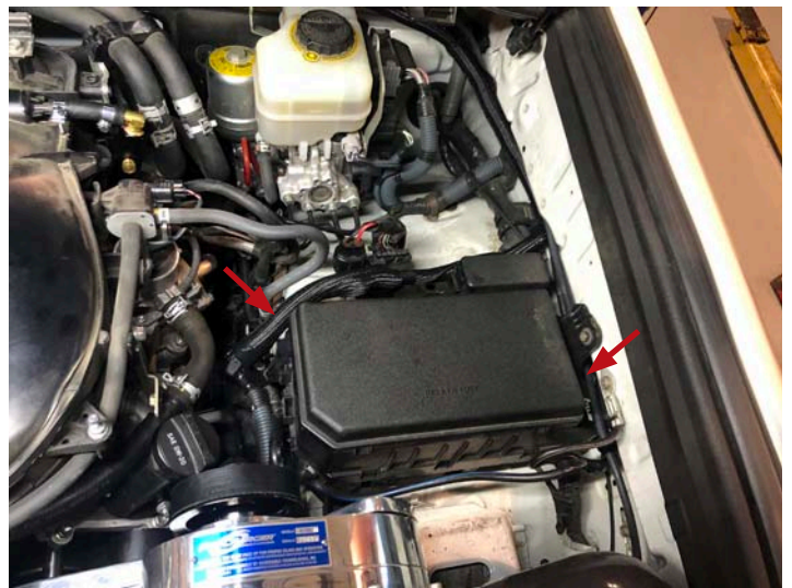
Route Cables Behind Fuse Box
