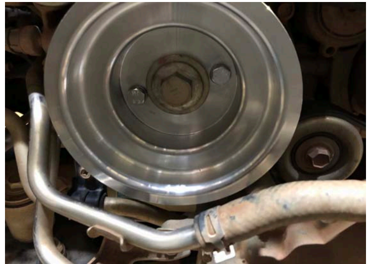
Crank Pulley Installed
