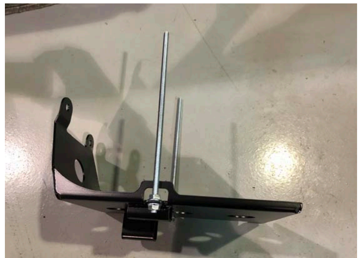
Studs Mounted To Battery Tray
