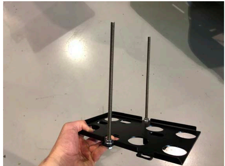
Studs Mounted To Battery Tray
