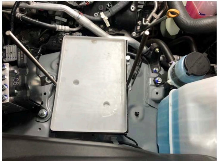
Plastic Battery Tray Installed
