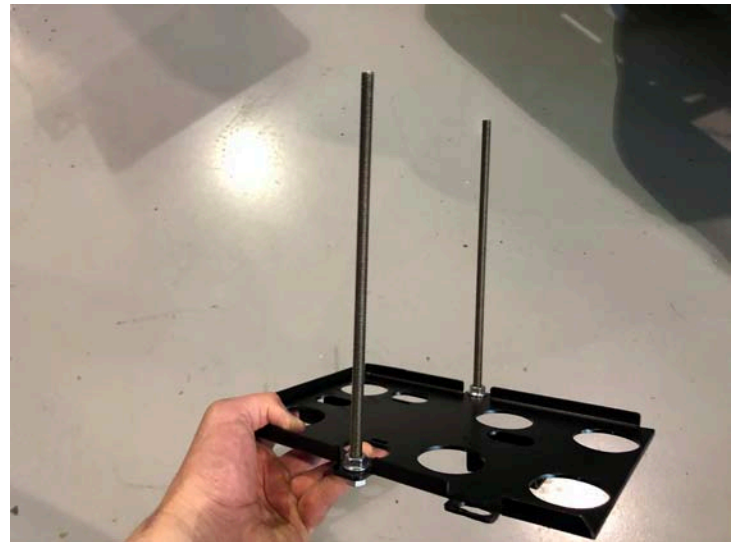
Studs Mounted To Battery Tray
