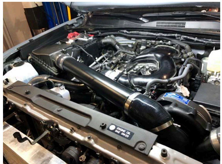
Air Inlet Tube Installed
