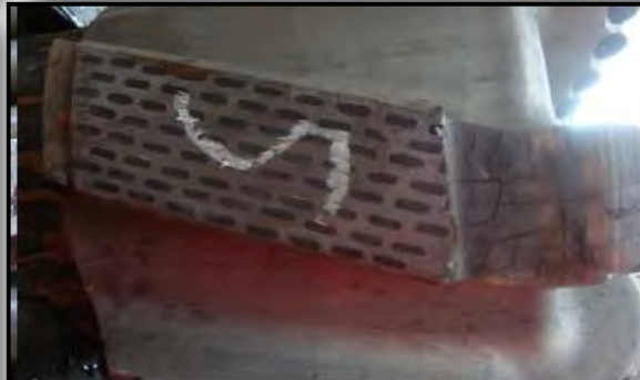
Blade 5- Shoulder is worn out
