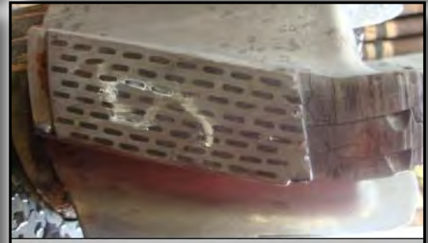
Blade 6- Shoulder is worn out
