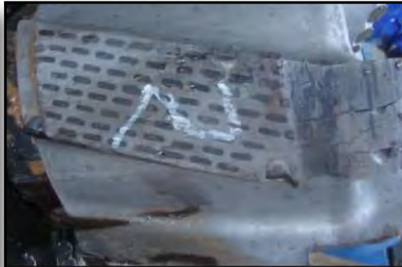
Blade 2- Shoulder is worn out
