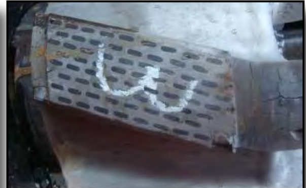
Blade 3- Shoulder is worn out
