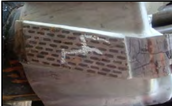
Blade 4- Shoulder is worn out
