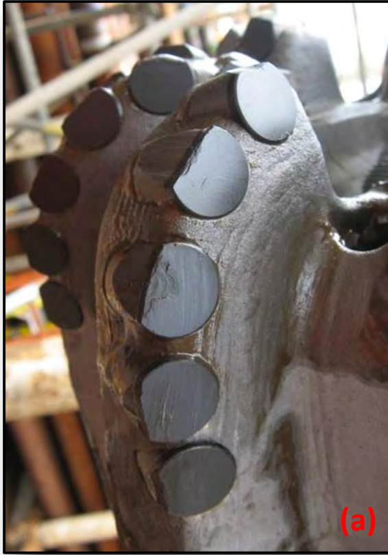
(a) Micro-spalls along wear flats - thermal; (b) Spalling of thermo-mechanical origin
