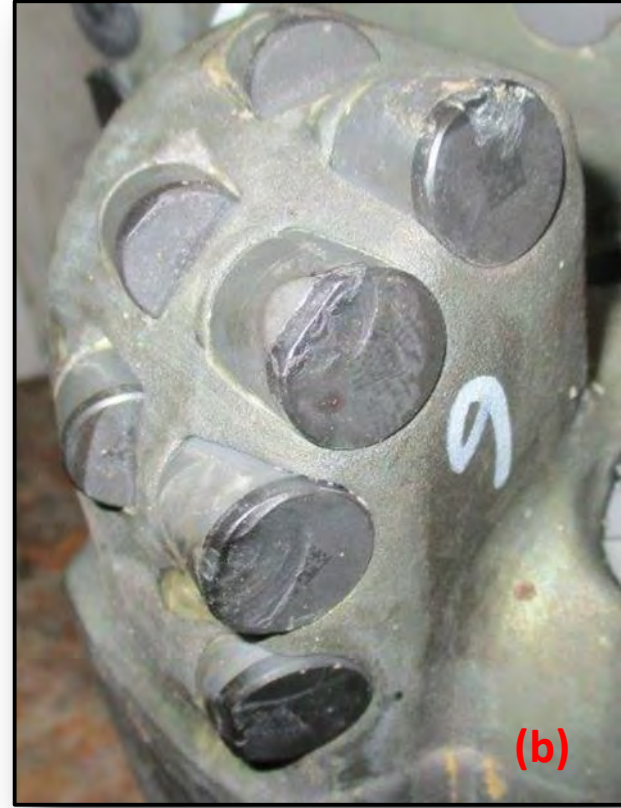
(a) Micro-spalls along wear flats - thermal; (b) Spalling of thermo-mechanical origin
