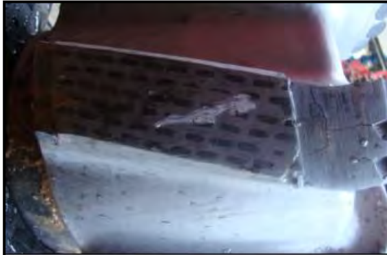
Blade 1-Shoulder is worn out
