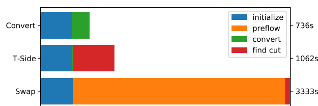
■ Figure 6 Distribution of spent time during Gusfield’s algorithm on the soc-slashdot instance with three approaches to use the Push-Relabel algorithm as a min-cut oracle. We split the measurements into initialization, preflow, conversion, and cut identification. The time overhead for measurement, logging, and the logic of Gusfield’s algorithm is included in the numbers on the right but excluded in the bars.
