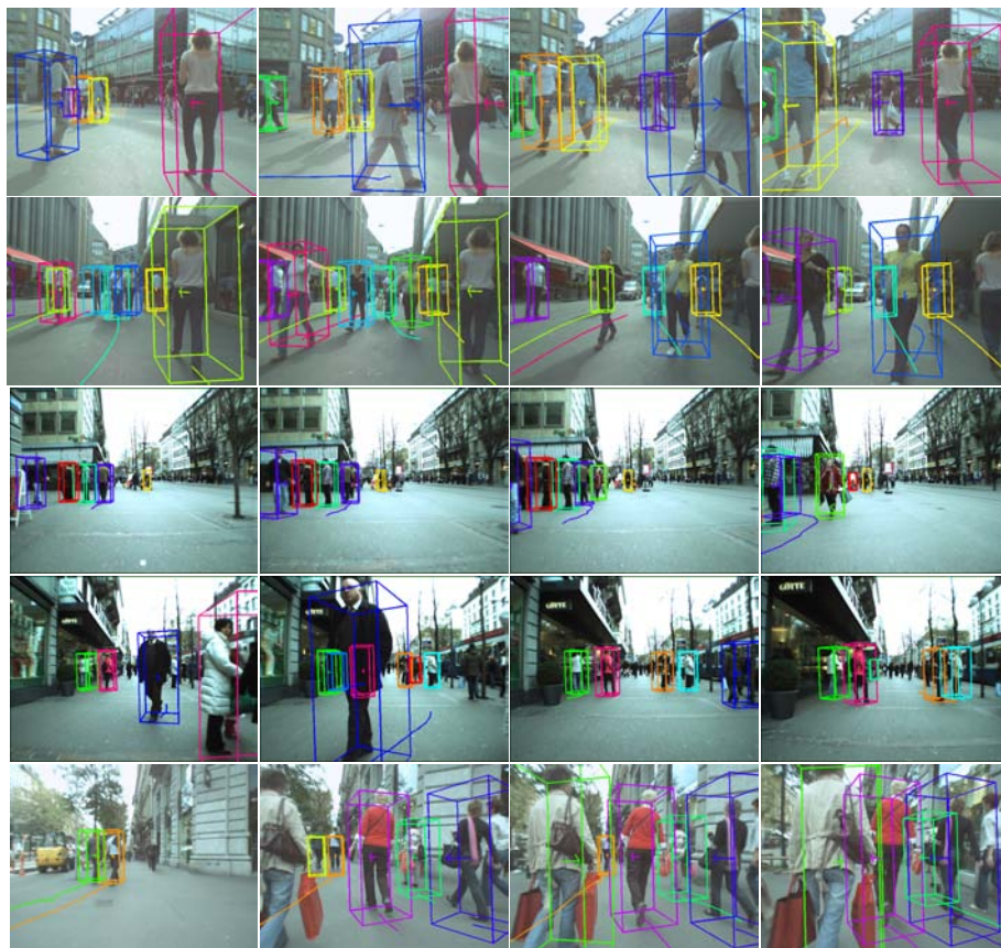
Fig. 9. Top two rows: exemplary subsequences from Seq.#2. Note the long trajectories and ability of the tracker to handle temporary occlusions in complex scenarios. Other rows: selected tracking results for Seqs. #3, #4, and #5.
