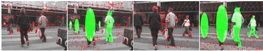
Fig. 4. Object detection and tracking give semantic meaning to the image and can be used to restrict localization efforts to parts that are believed to be static.
