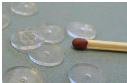
Fig. 8: Replicated PMMA parts with microstructures.
