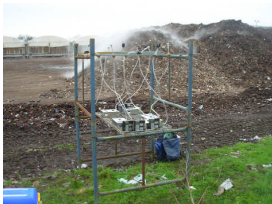
Fig. 1. The two types of samplers with the pumps and sampling boxes on the lower platform for easy access, and the sampling heads at the end of the tygon tubing at a height of 1.8 m. The compost windrow can be seen in the background.
