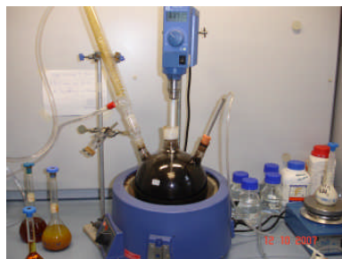
Fig 1. Dispersing of ferrite nanoparticles and embedding them in a three neck flask under nitrogen. The displacement of air by N 2 gas during preparation prevented oxidation of ferrous ion in the aqueous solution and also controlled the particle size.
