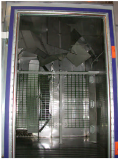
Figure 2. Internal view of the reverberation chamber showing the two stirrers.
