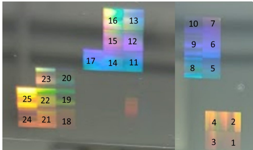
Figure 4: The output of 25 different gratings where the first of each set is a single layer and the layers increase as the number value increases. The spacing in each set is altered between layers. Sets 1-4 have 8\ \mu\text{m} layer separation, 5-10 have 10\ \mu\text{m} layer separation, 11-17 have 15\ \mu\text{m} separation and 18-25 have 20\ \mu\text{m} separation.
