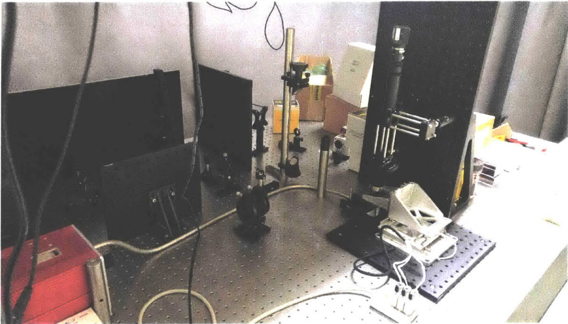
Figure 46: Setup for femtosecond laser micromachining.
