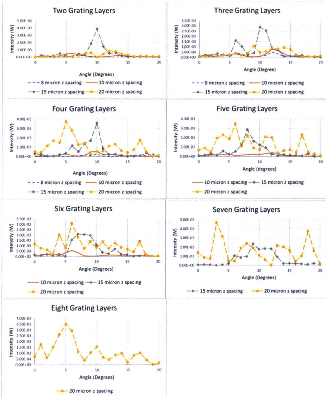
Figure 78: Adapted from [50]. Angular characterization of multilayer gratings fabricated in glass.
